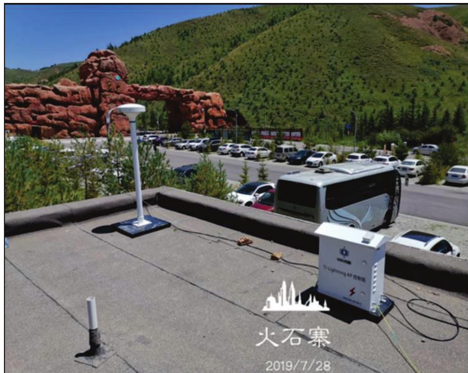
Figure 2-5 Pictures of fast antennas and controlling box.
