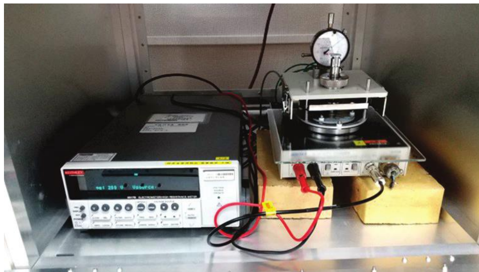
Fig.2.13 Photographic image of RT resistance measurement system with a resistivity chamber inside a Faraday cage.
