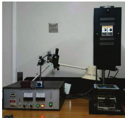
Fig.2.15 Photographic image of a solar simulator used in this study.
