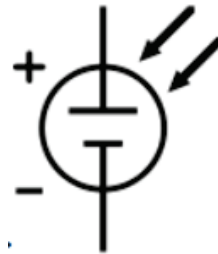
Fig.1.5 The schematic symbol of a solar cell.
