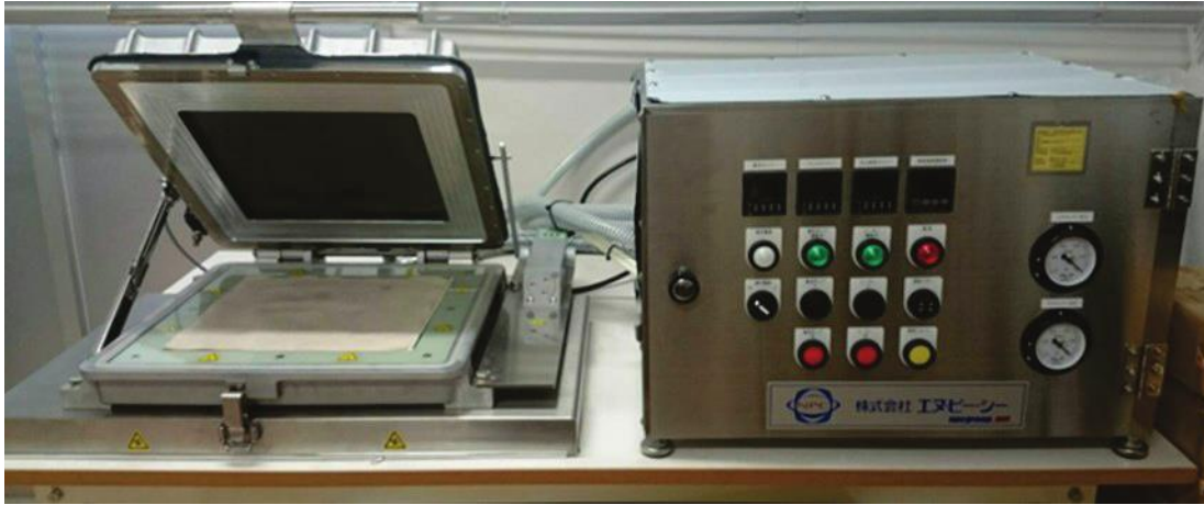
Fig.2.2 Vacuum Laminator (left chamber, right: operation panel).
