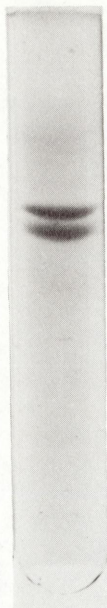
Fig. 5. SDS-Polyacrylamide gel electrophoresis. The purified preparation was treated with SDS and 2-mercaptoethanol as described in "Experimental Procedure" and an aliquote ( 3\mu\text{g} in 0.15 ml of the reaction mixture) was subjected to electrophoresis. A constant current of 8 mA per gel was applied for 4.5 hrs. The concentration of acrylamide in the gel was 10%.
