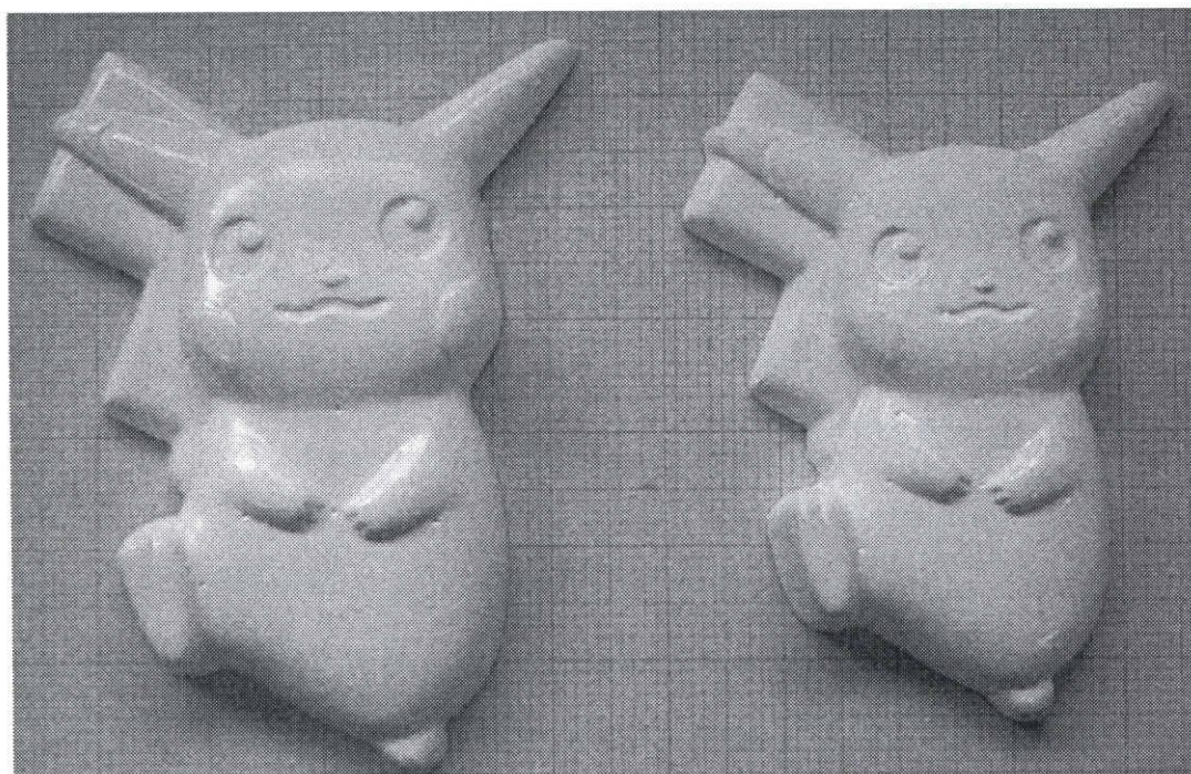
Fig. 3-4-7 A intricate green body ( left ) and the sintered body ( right ).
