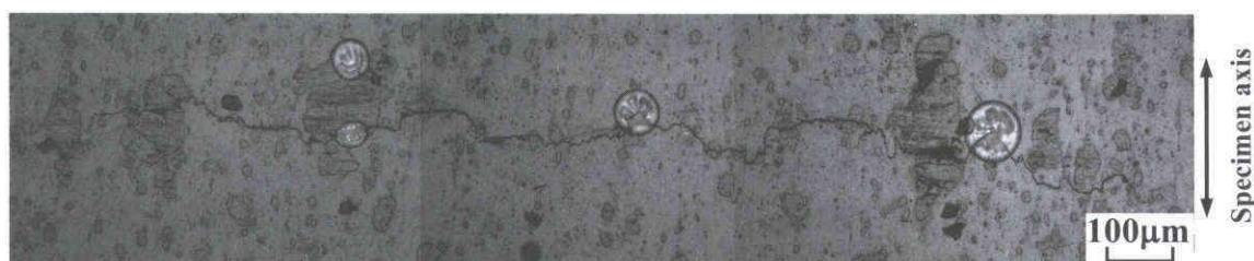
Fig.6-15 An example of small crack growth path ( Mg_2Si -F, \sigma=100MPa ).
