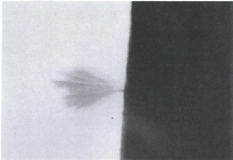
(a) 内導トリー (525 \mu\text{m} ) (a) vented tree which grew from inner semiconducting layer
