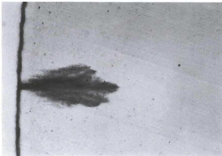
(b) 外導トリー (950 \mu\text{m} ) (b) vented tree which grew from outer semiconducting layer
