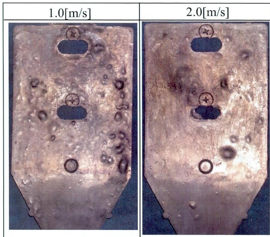
Fig. 3.2 Results of a brister test ( v_\ell = 0.5[\text{m/s}] , v_h = 1.0, 2.0[\text{m/s}] )
