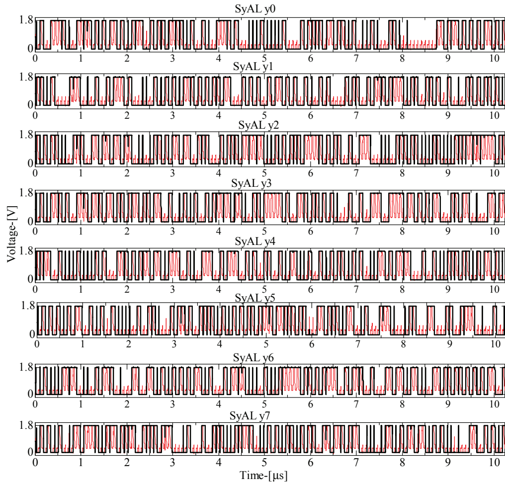
Figure 5.38: Output voltage of the SyAL S-box at 12.5 MHz power clock frequency.
