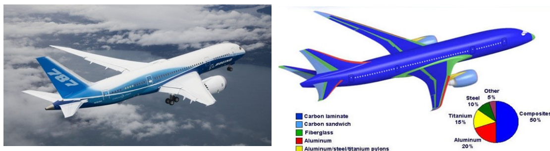
Fig. 1.1 Examples of CFRP applications for aircrafts
