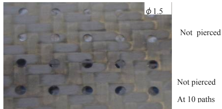
Fig.3.16 Example of before piercing and after piercing (CFRTP thickness 0.5mm, 1.5mm dia., after 10 paths)
