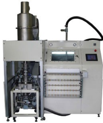
Fig.3.3 Picture of a blast machine (Elfo-blaster ELP-3TR)
