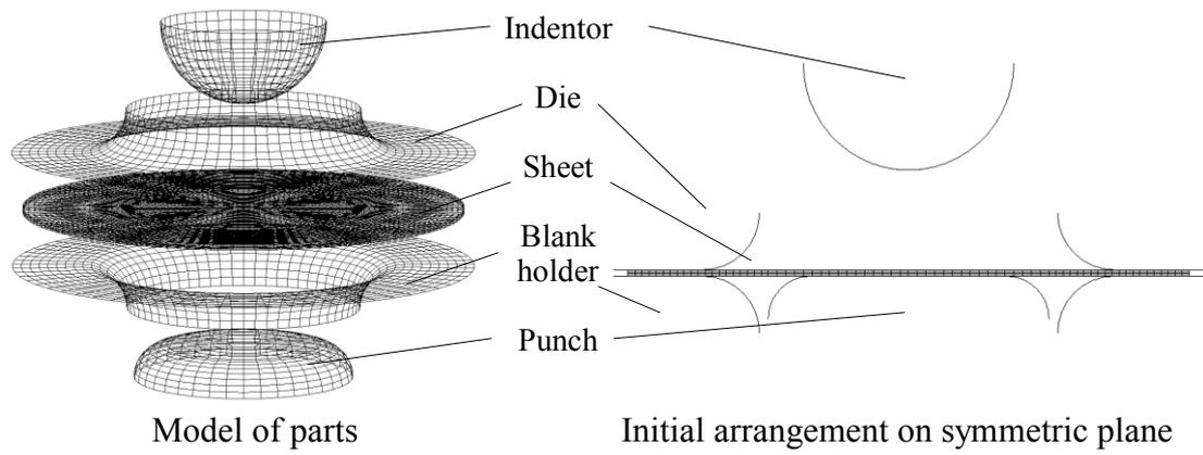
Fig. 2.8 Numerical model (FS: Flat top shell and hemispherical indenter).
