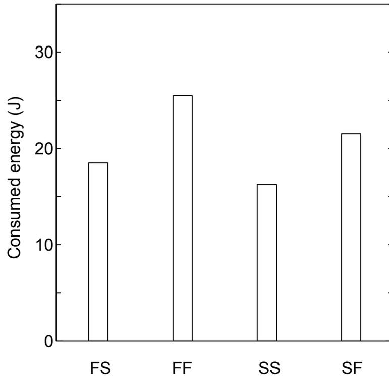
Fig. 2.7 Summary of consumed energy in indentation stroke equal to shell height.
