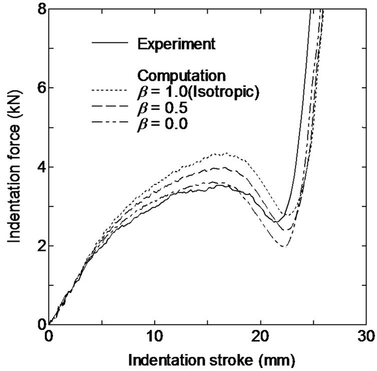
Fig. 2.13 Indentation force – strokes curves for isotropic or kinematic hardening property.
