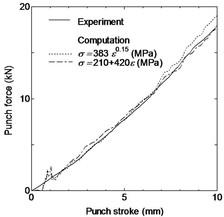
Fig. 2.12 Punch force – stroke curves in computation for two mechanical properties.
