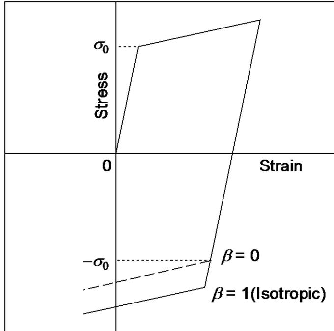
Fig. 2.11 Kinematic linear hardening plasticity.
