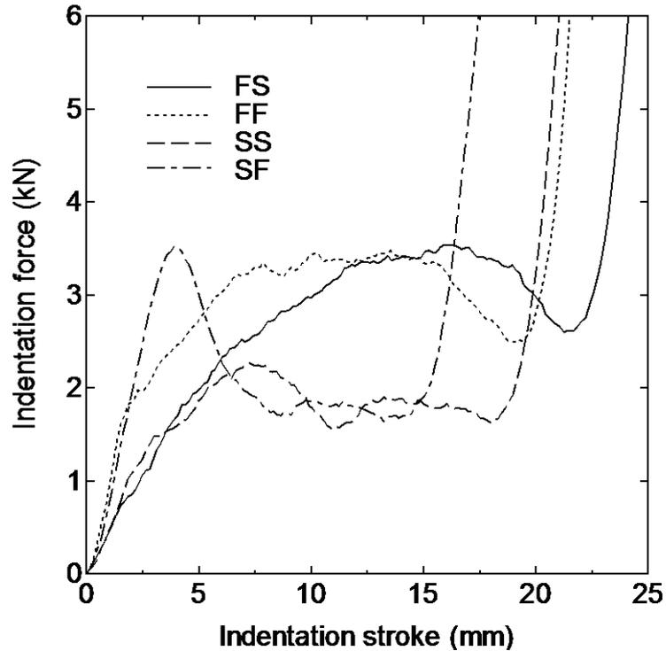
Fig. 2.5 Indentation force curves under various indentation conditions.
