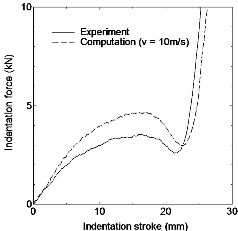
Fig. 2.10 Indentation force-stroke curves in FS.
