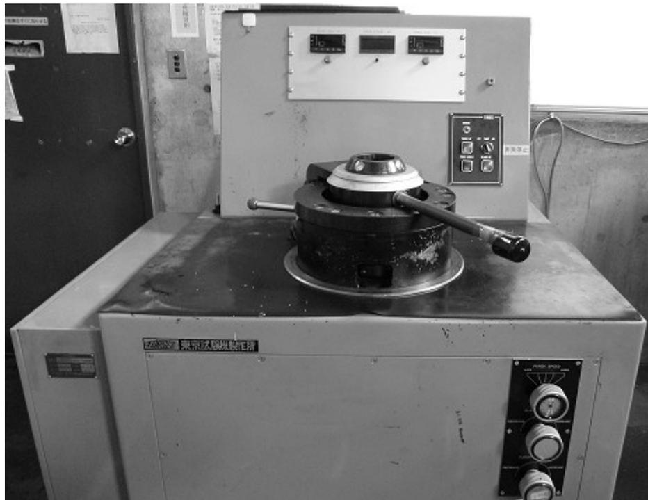
Fig. 2.1 Hydraulic-type deep-drawing testing machine
