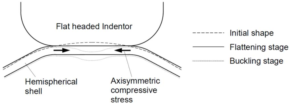
Fig. 2.6 Deformation behavior in early indentation stage of SF.
