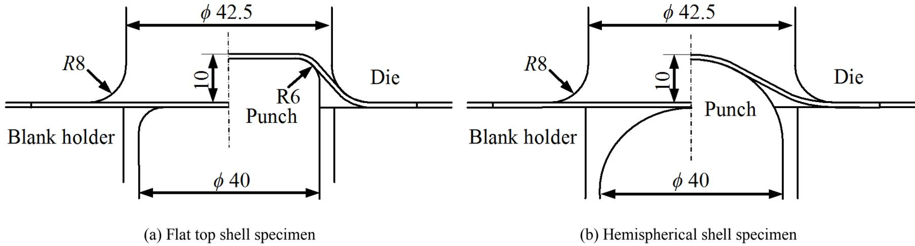
Fig. 2.2. Sheet drawing process.
