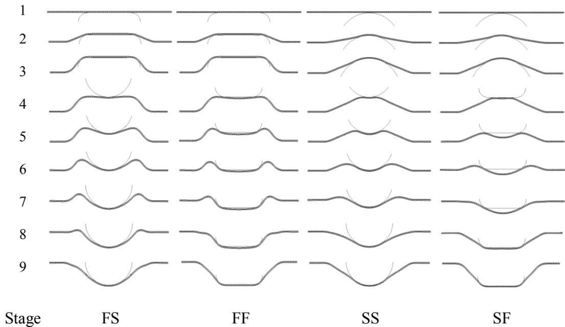
Fig. 2.14 Progressive deformation patterns in computation, Stage 1 ~ 3: Forming process, Stage 4 ~ 9: Indentation process, Indentation stroke: 1, 5, 10, 15, 20, 25 mm (Stage 4 ~ 9).
