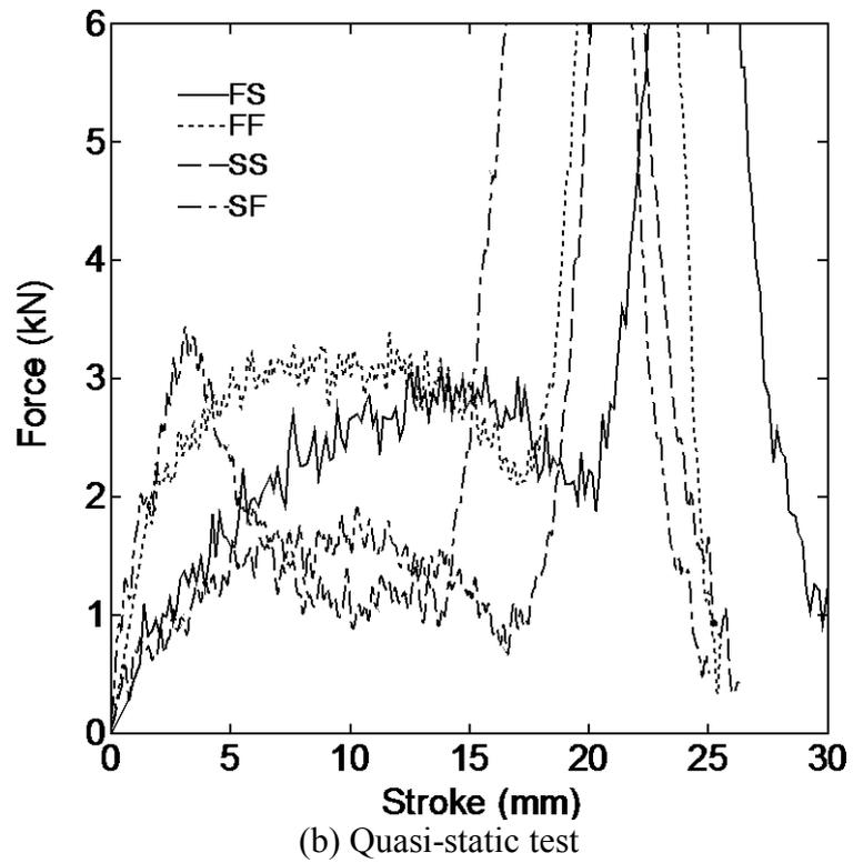
Fig. 3.6. Force curves for flat top and hemispherical top shells of aluminium alloy.
