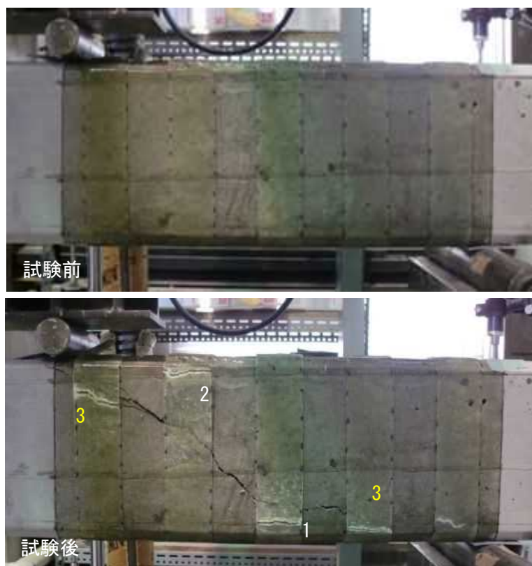
写真-3.10 No. 9 (50% 90 度) せん断破壊状況
