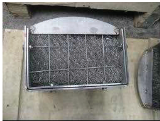
Fig.2-14 Demister mounting situation
