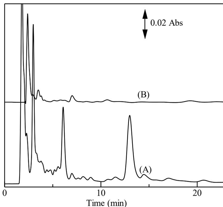
Fig. 2-4 Effect of urea on on-line BSA digestion in the immobilized-enzyme microcolumn (100 x 0.32 mm I.D) (A) with urea (B) without Urea. Condition: mobile phase, 0.1 mol/L Tris-HCl buffer (pH 8.3) with flow rates 3  $\mu\text{L}/\text{min}$  for separation and flow rate 1  $\mu\text{L}/\text{min}$  for digestion. Separation column: L-column2 ODS (100 x 0.32 mm I.D). Digestion system monitored at 214 nm.
