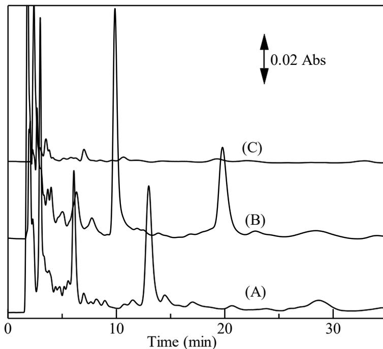
Fig. 2-7 Chromatograms of the injection of BSA in the immobilized-enzyme microcolumn (100 x 0.32 mm I.D.). Digestion system monitored at 214 nm. The experiment was conducted with 0.1 mol/L Tris-HCl buffer solution pH (A) 8.3 (B) 7.3 (C) 5.4 with flow rate for separation 3  $\mu$ L/min and flow rate for digestion 1  $\mu$ L/min. Separation column: L-column2 ODS (100 x 0.32 mm I.D.)
