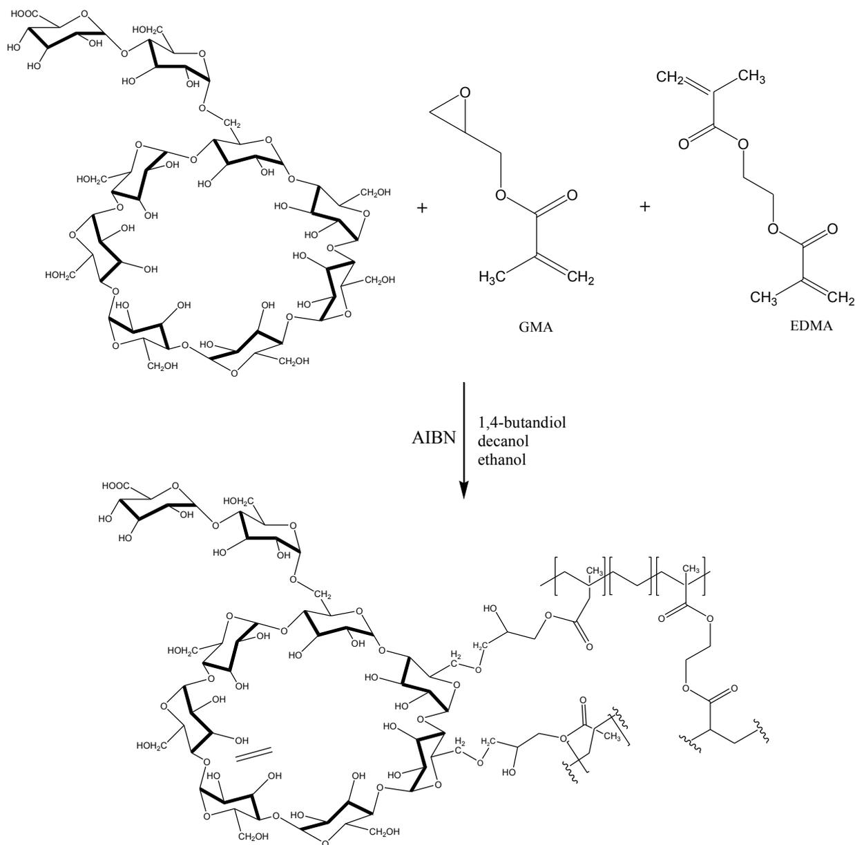
Fig. 3-1 Schematic diagram for chiral stationary phase preparation
