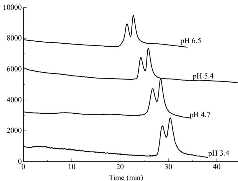
Fig. 3-6 The influence of pH on retention of Dansyl-DL-threonine. Conditions: column, 100x0.32 mm I.D.; mobile phase, ACN/60 mM AMAC buffer (pH 4.7) 30/70 (v/v); flow rate, 1 $\mu$ L/min; wavelength of UV detection, 254 nm; column temperature, 20 $^{\circ}$ C.
