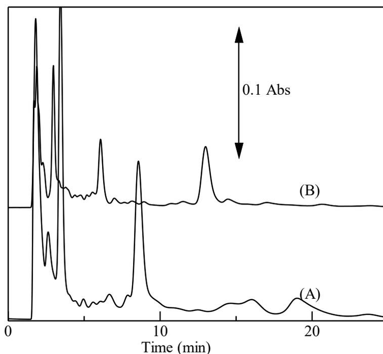
Fig. 2-6 Chromatograms of the injection of BSA in the immobilized-enzyme microcolumn (100 x 0.32 mm I.D.). Digestion system monitored at 214 nm. The experiment was conducted with (A) 0.1 mol/L Tris-HCl buffer solution (pH 8.3) (B) 0.1 mol/L phosphate buffer solution (pH 8.1) with flow rate for separation 3  $\mu\text{L}/\text{min}$  and flow rate for digestion 1  $\mu\text{L}/\text{min}$ . Separation column: L-column2 ODS (100 x 0.32 mm I.D.).
