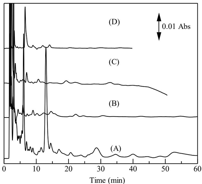
Fig. 2-5 Effect of the sample flow rate on on-line BSA digestion in the immobilized-enzyme microcolumn (100 x 0.32 mm I.D). Condition: mobile phase, 0.1 mol/L Tris-HCl buffer (pH 8.3) with flow rates of digestions (A) 1 (B) 2 (C) 3 and (D) 4  $\mu\text{L}/\text{min}$  and separation flow rate 3  $\mu\text{L}/\text{min}$ . Separation column: L-column2 ODS (100 x 0.32 mm I.D). Digestion system monitored at 214 nm.
