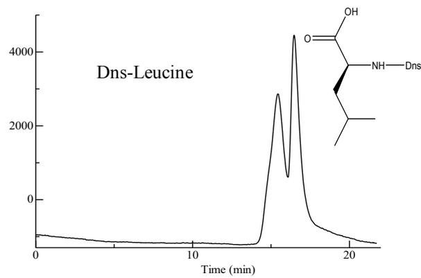
Fig. 3-5 Chromatograms of the separation of chiral analytes with mixture of ACN/60 mM AMAC buffer (pH 4.7) 30/70 (v/v). Conditions: column, 100x0.32 mm I.D.; flow rate, 1 $\mu$ L/min; wavelength of UV detection, 254 nm.
