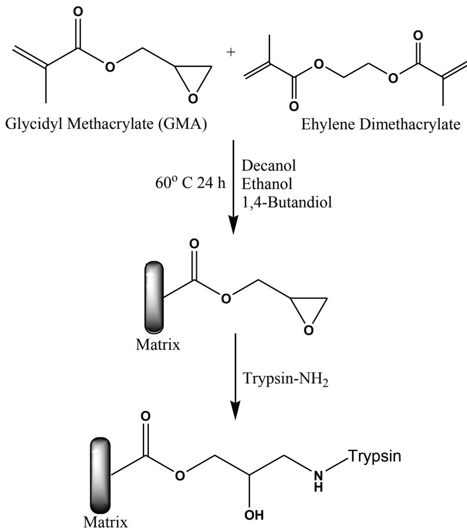
Fig.2-1 Schematic diagram for IMERs preparation
