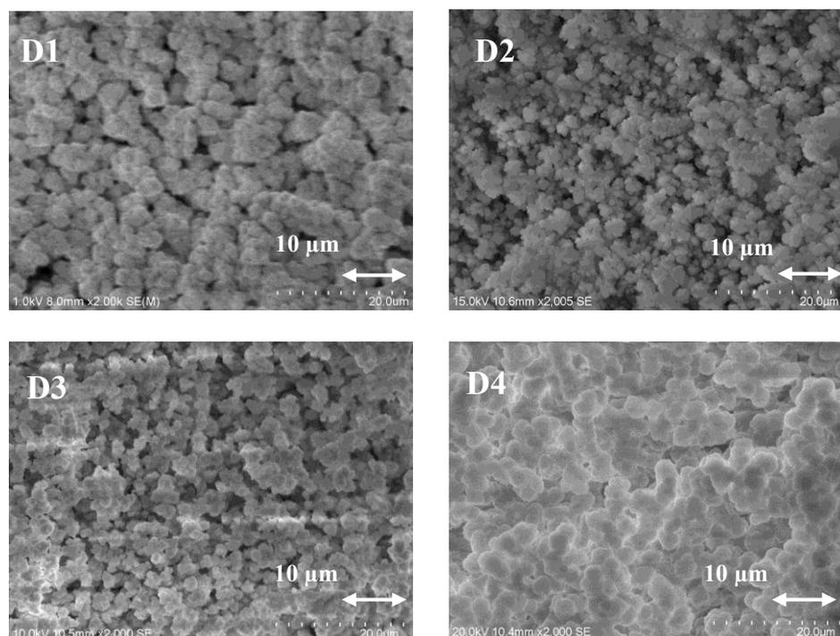
Fig. 2-2 Scanning electron microscopy of the internal structure of monolith in the capillary(magnification 2000x).
