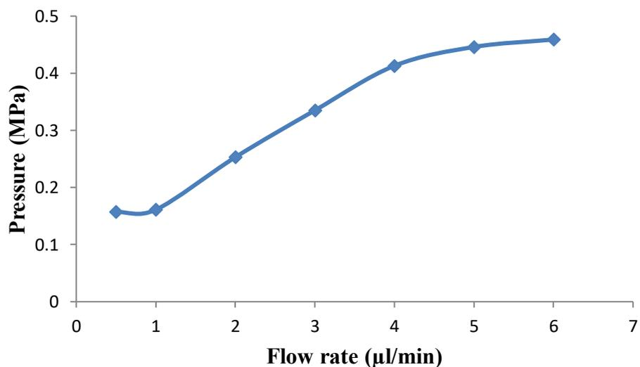
Fig. 3-2 Effect of the flow rate on backpressure. Condition: mobile phase, ACN/100 mM TEAA (pH4.1) 30/70 (v/v). Chiral stationary phase column: 100 x 0.32 mm I.D.
