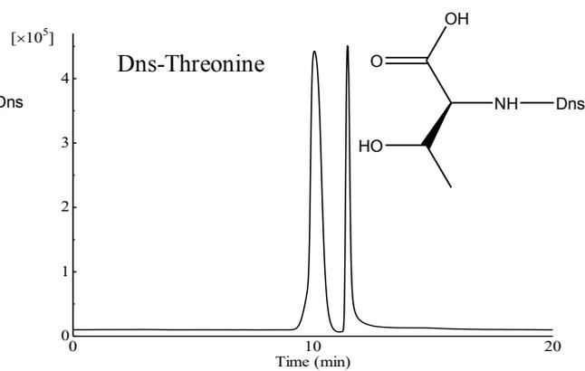
Fig. 3-4 Chromatograms of the separation of chiral analytes with mixture of ACN/100 mM TEAA buffer (pH 4.1) 30/70 (v/v). Conditions: column, 100x0.32 mm I.D.; flow rate, 1 $\mu$ L/min; wavelength of UV detection, 254 nm.
