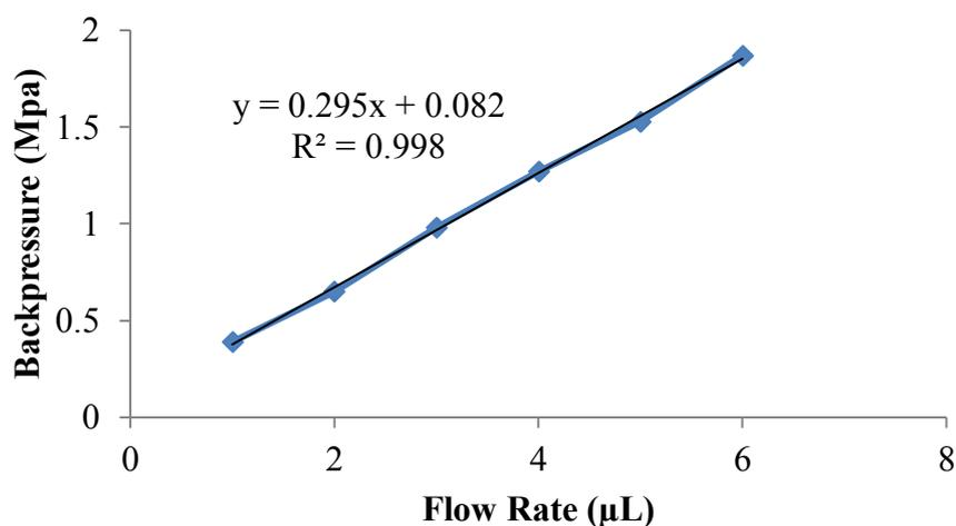
Fig. 2-3 Effect of the flow rate on backpressure. Condition: mobile phase, 0.1 mol/L Tris-HCl buffer. Immobilized column : 100 x 0.32 mm I.D.
