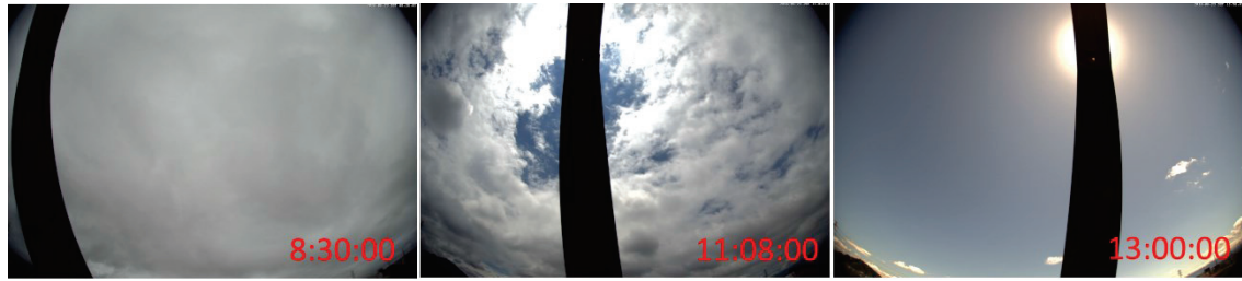
Fig. 5.2 Cloud images taken by sky camera, the black bands in them are shadow blades.
