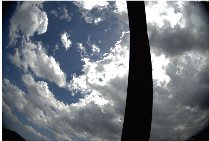
Fig. 3.4 Cloud image when solar irradiance changed suddenly; Taken by sky camera, the black band in it is the shadow blade. (April 17, 2016. 13:07)
