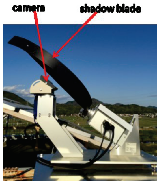
Fig. 2.7 Sky camera with shadow blade
