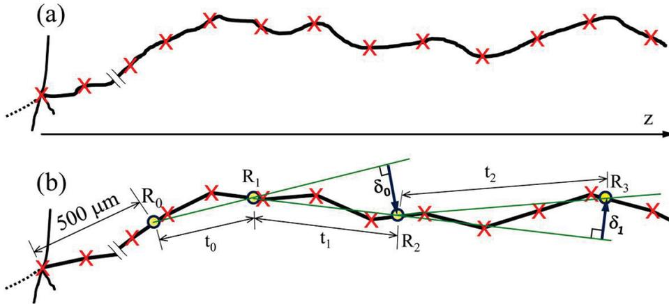
Fig. 3.2. A schematic drawing of  $\sigma$ -stop counting by a negative particle from the right
