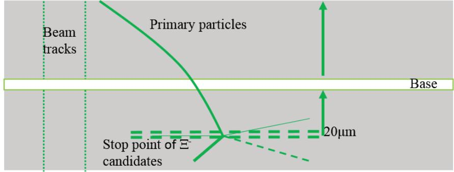
**Fig. 3.3** Sketch of measurement of multiple coulomb scattering
