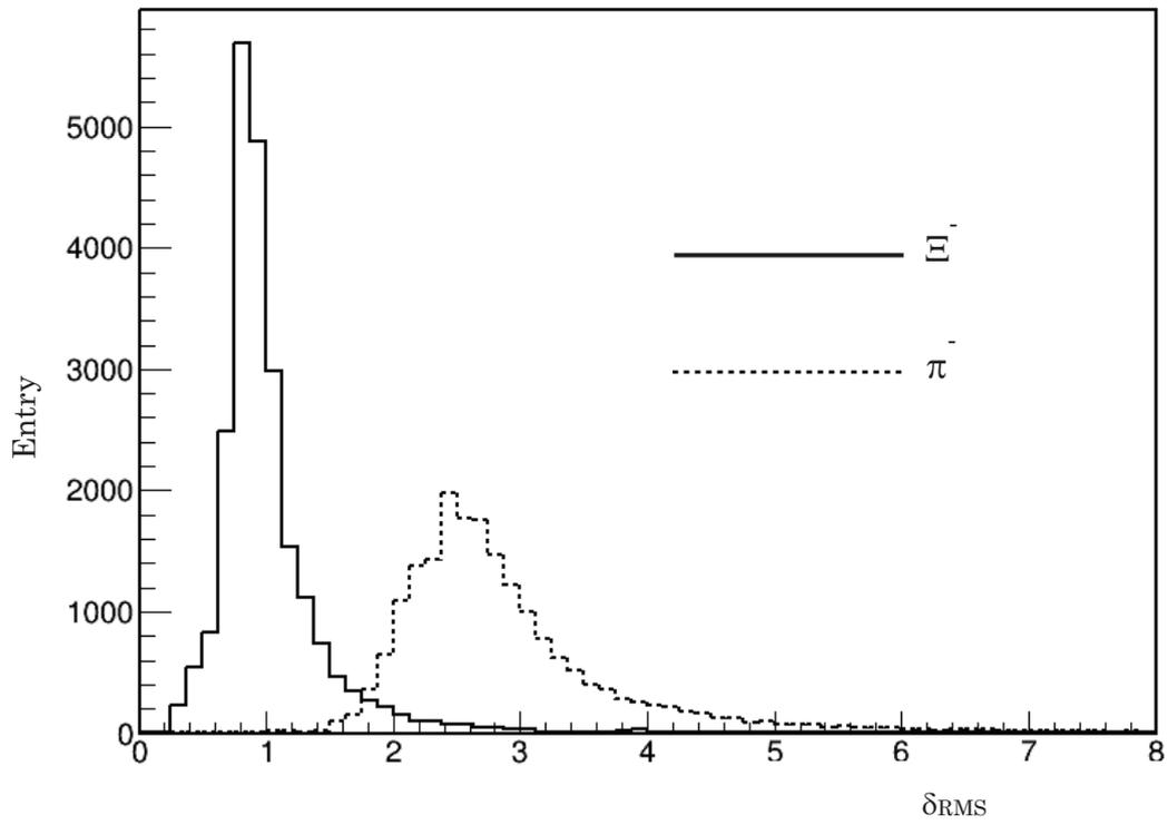
Fig 3.7 RMS of the second difference of revised data samples with measurement errors for  $E^-$  and  $\pi^-$  produced by Geant4 package.
