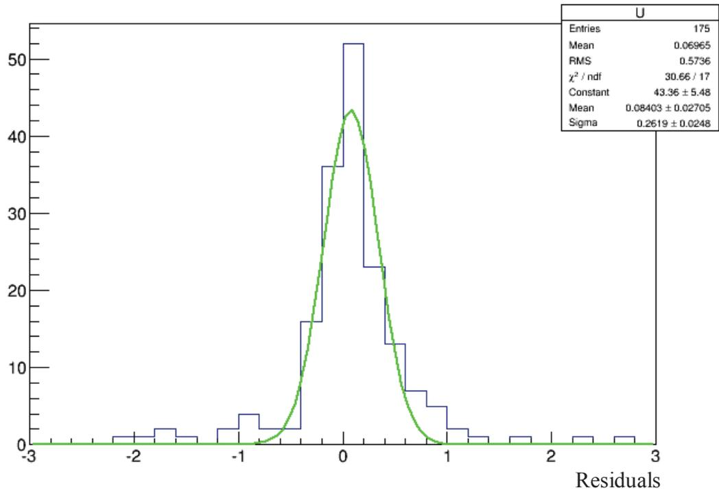
**Fig. 3.5 (b).** Obtaining measurement error of Y components from Gaussian fitting of residuals Distortion Correction by using beam tracks
