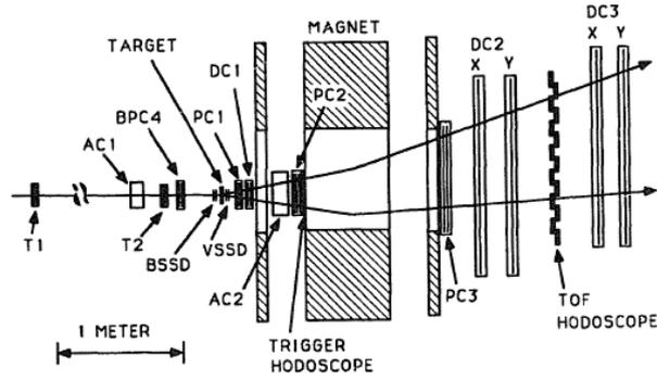
Fig 2.1 Experimental Setup of KEK-E176 experiment
