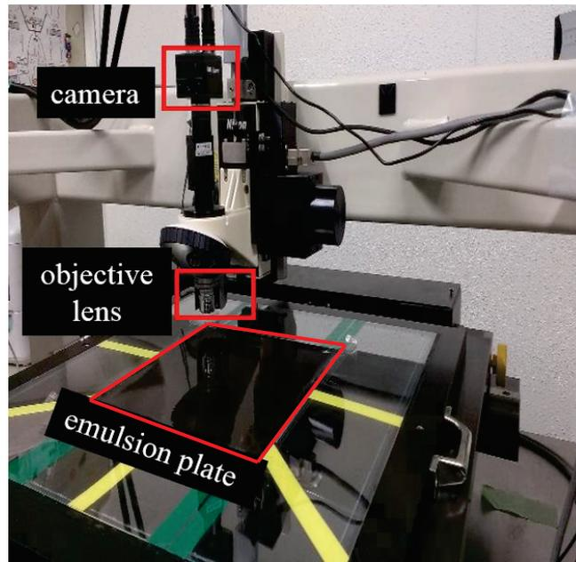
Fig. 2.4 An optical microscope system
