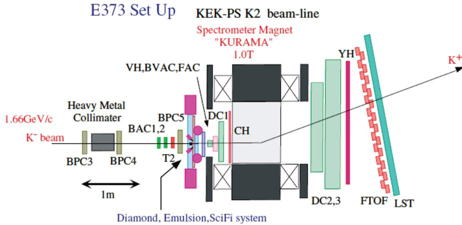
Fig 2.2 Experimental Setup of KEK-E373 experiment
