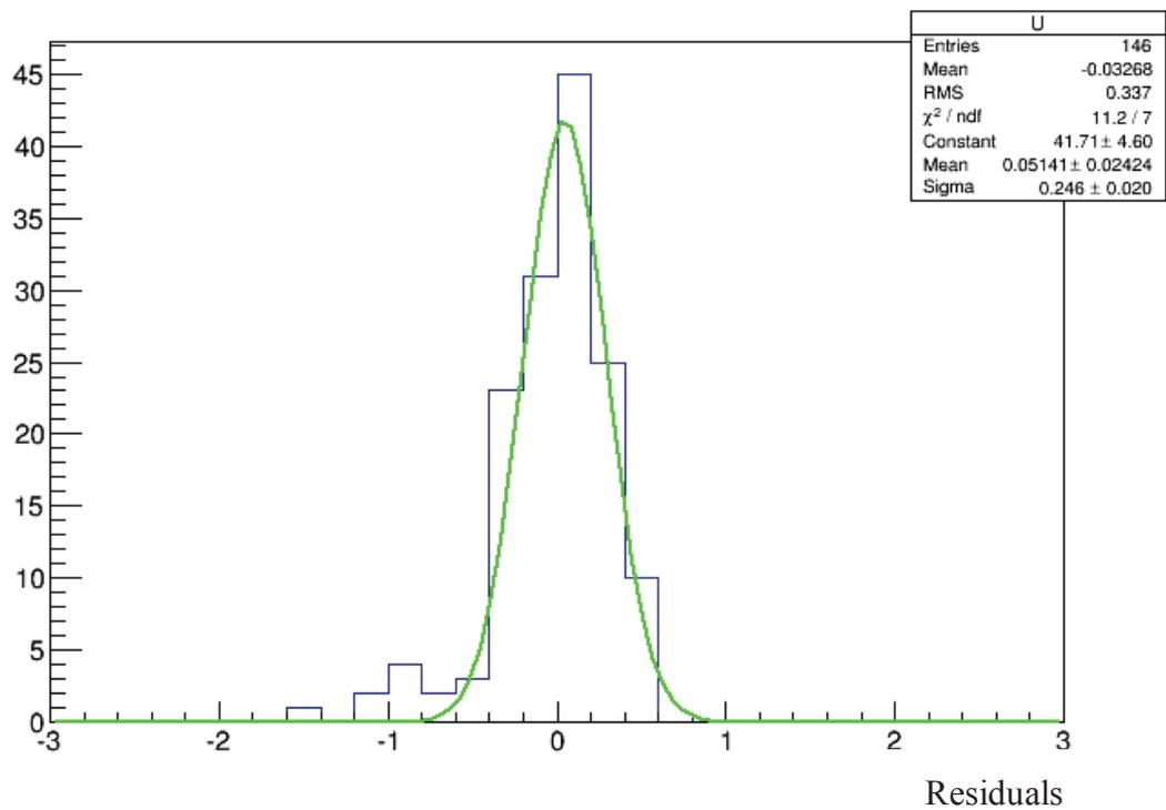
Fig 3.5 (a). Obtaining measurement error of X components from Gaussian fitting of residuals Distortion Correction by using beam tracks
