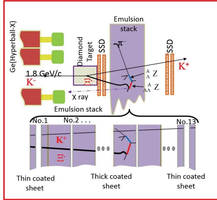
Fig 2.3 Experimental Setup of KEK-E373 experiment
