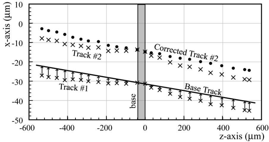
**Fig. 3.4** Distortion Correction by using beam tracks
