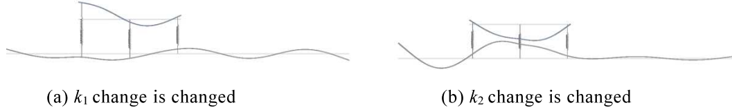
Fig. 4-8 Eigen mode shapes at 250Hz in case of k_1, k_2 change.
