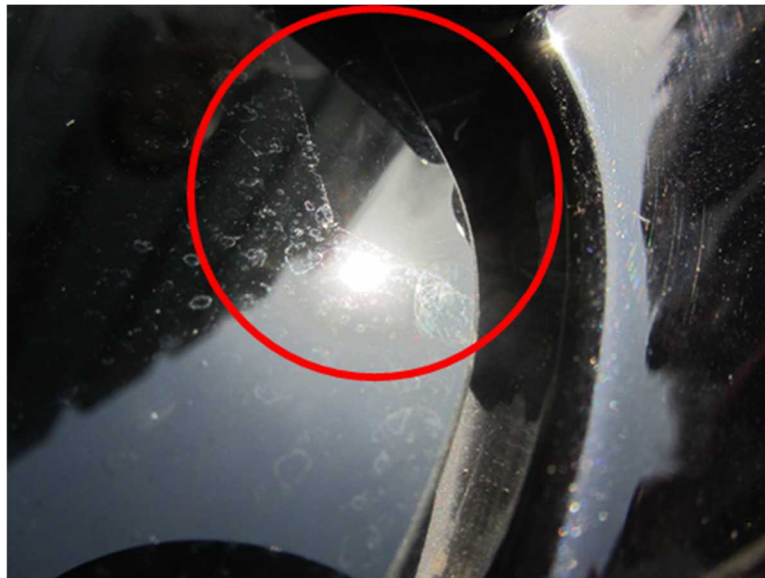
Fig. 6-11 Removal of ring deposits on the rear glass of an actual vehicle by 0.5% HF
