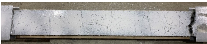
Figure 2.15 – Crack pattern of TR-SHCC specimens
