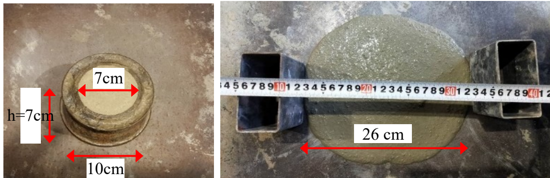
Figure 2.5 – Flow test to determine flow diameter of mortar
