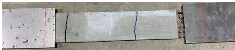
Figure 2.13 – Crack pattern of TRC-LS specimens made of low strength ordinary mortar
