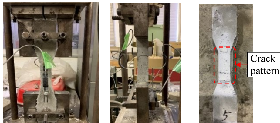
Figure 2.6 – Test setup and crack pattern of SHCC specimen
