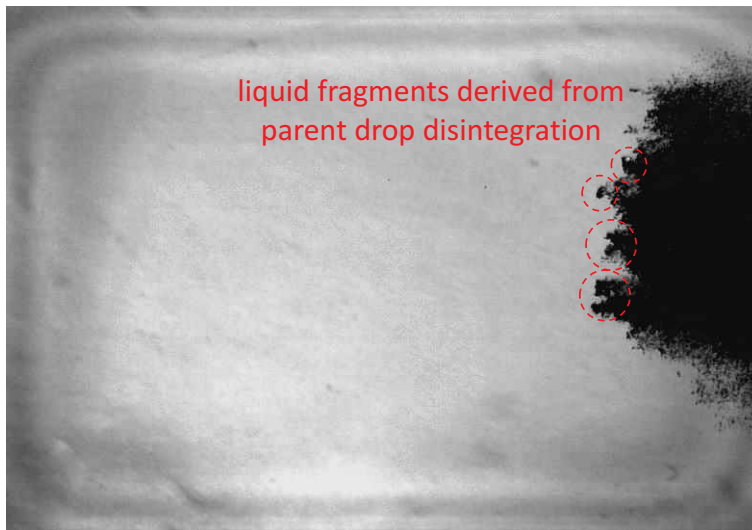
(b) liquid fragments derived from parent drop disintegration
