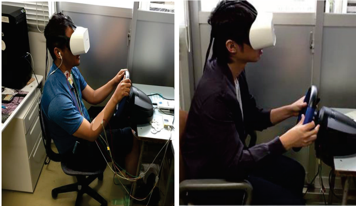
a) 3DVR and EMG recording setup
