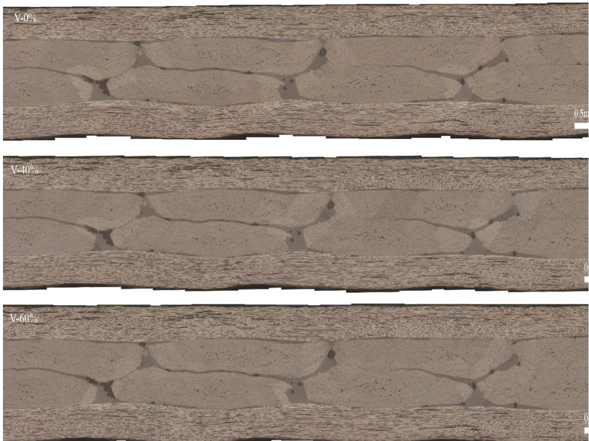
Fig. 9 Micrographic edge scanning of damage evolution corresponding to different loading stages on the load-displacement curve of the NM specimen.
