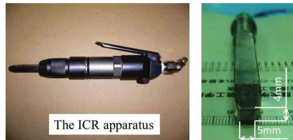
Figure 4-12 The ICR apparatus [21]
