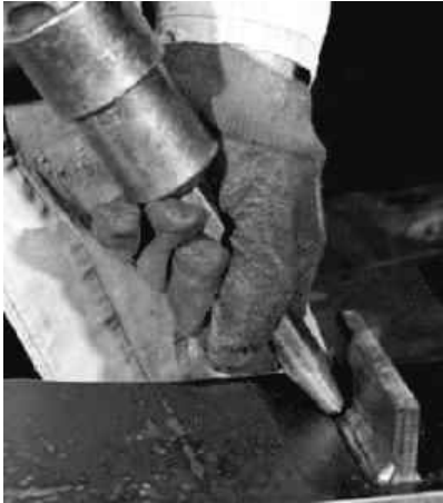
a Classical hammer peening [14]
