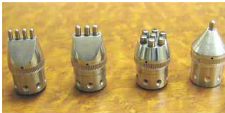
Figure 2-6 Examples of four different HFMI devices [28]
