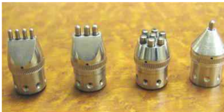
Figure 2-7 Examples of tip geometries and multiple indenter [29]
