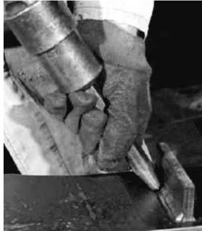
a Classical hammer peening [14]
