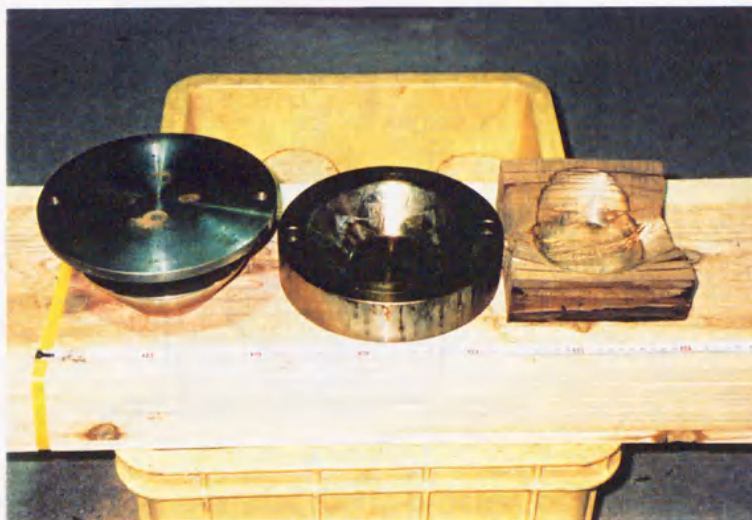
Fig. 1-23. The jig for manufacturing wooden bowl by compressive-molding under high temperature steam atmosphere.
