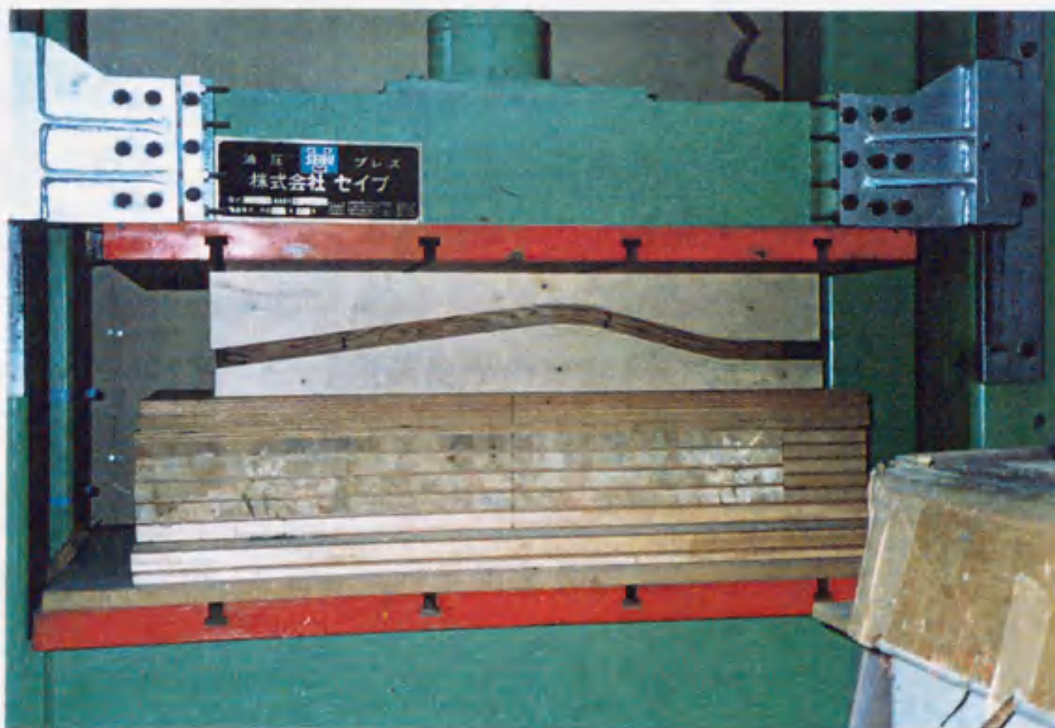
Fig. 3-9. The bending of Mizunara specimen.
