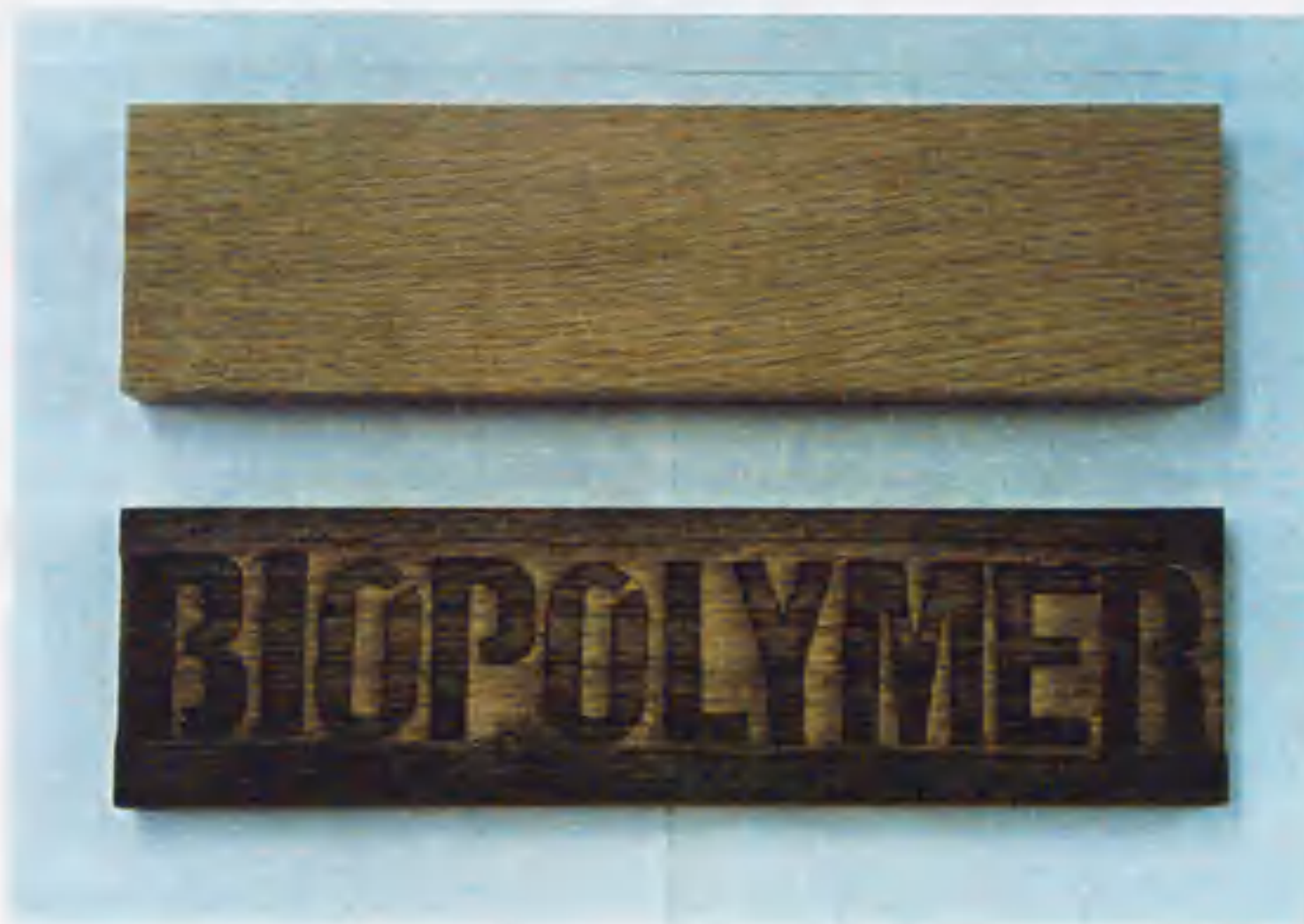
Fig. 1-18. Lumber transcribed the letter by compressing under high temperature steam atmosphere.
