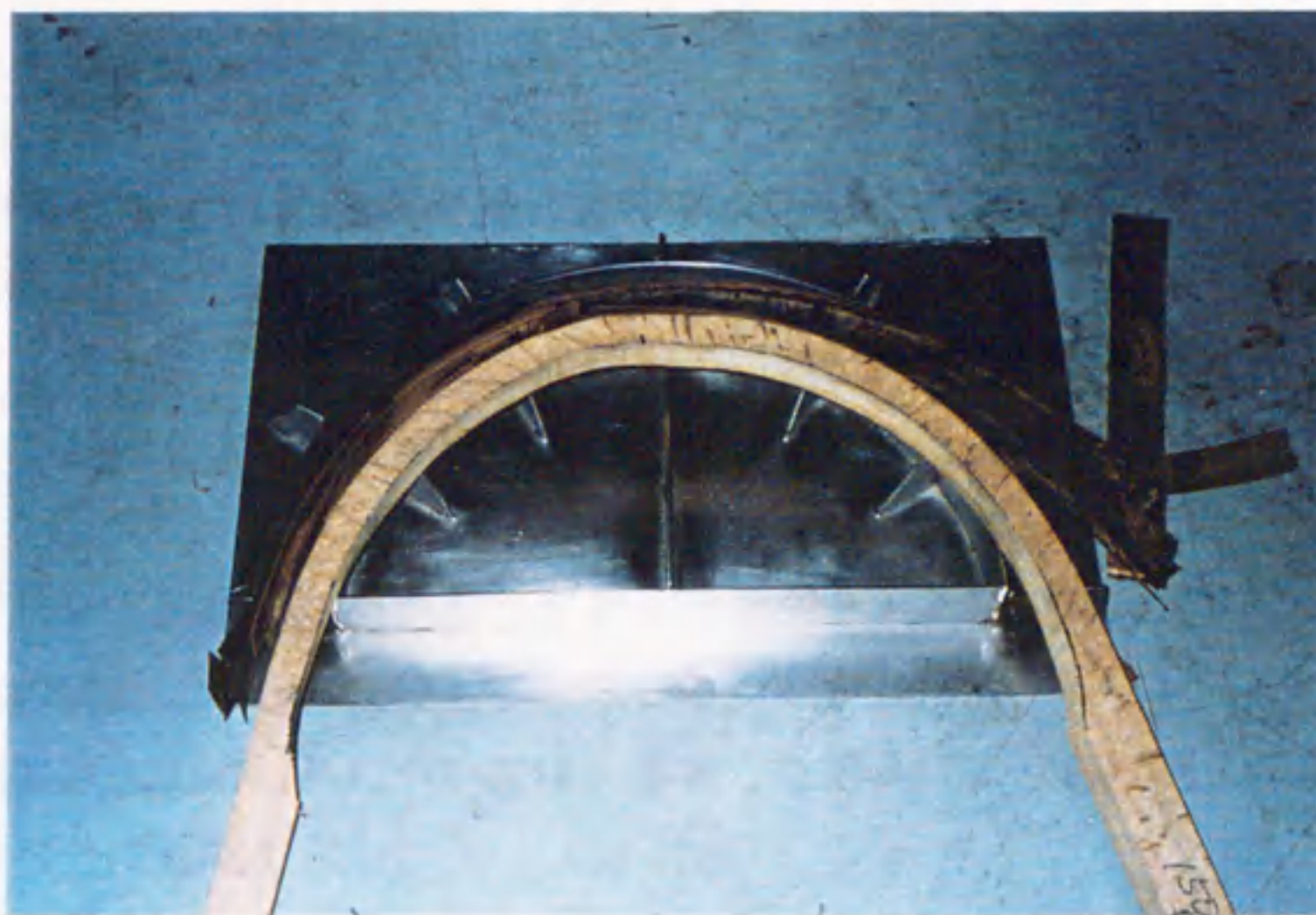
Fig. 3-20. The special-jig to fix the bending shape.
