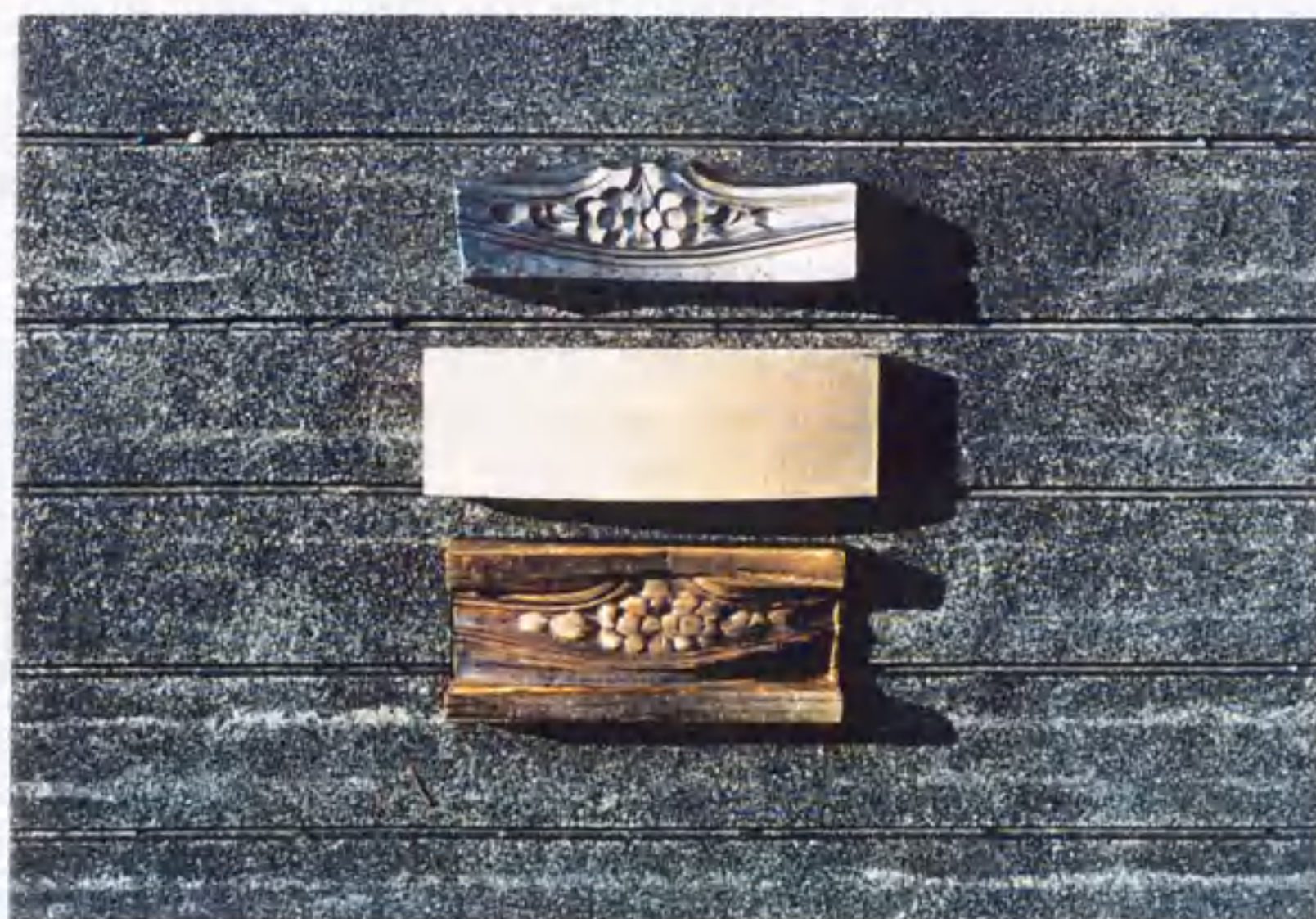
Fig. 1-20. The jig and relieves manufactured by compressive-molding under high temperature steam atmosphere.
