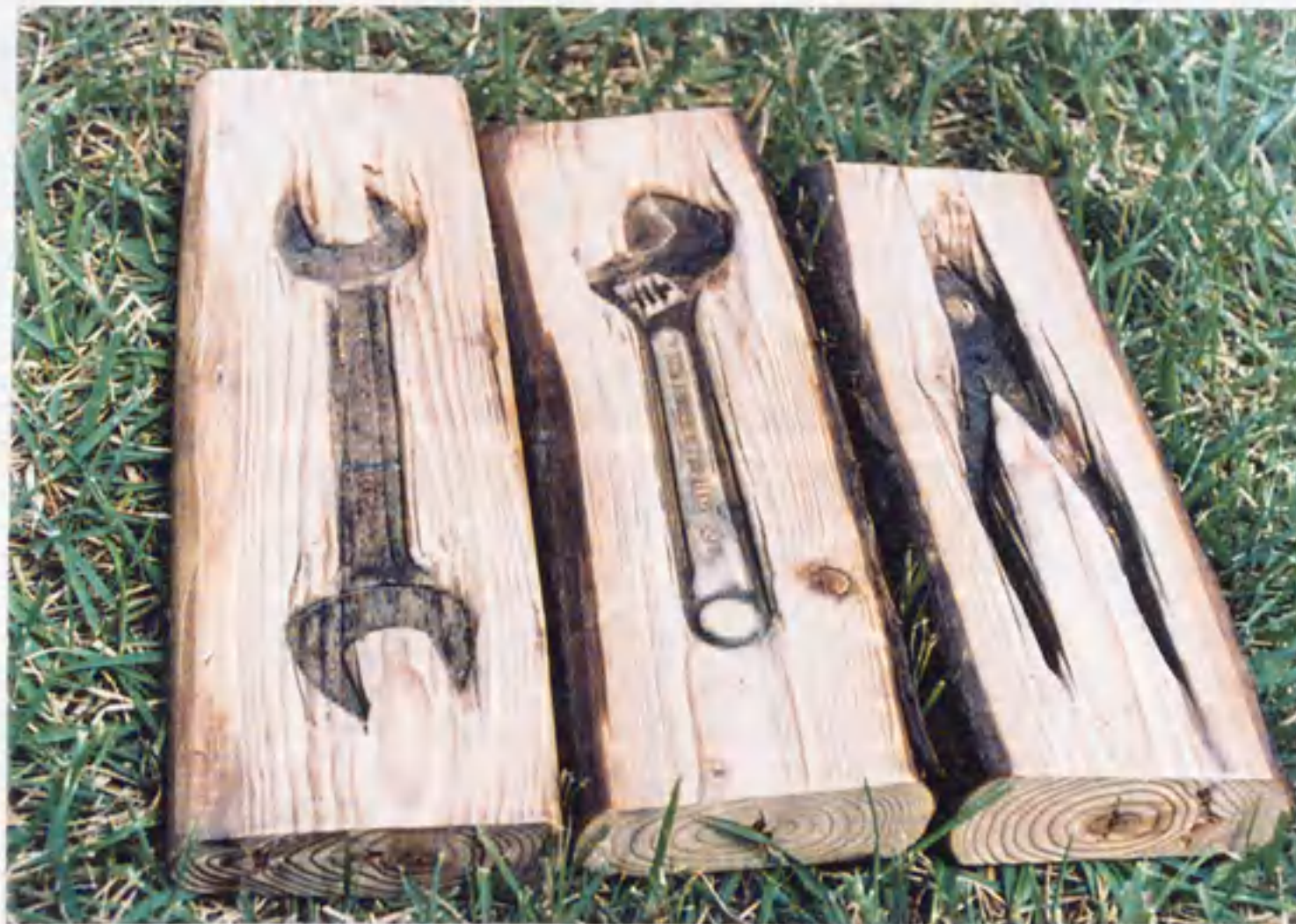
Fig. 1-17. Two-faced sawn lumber transcribed the shape of metal tool by compressing under high temperature steam atmosphere.
