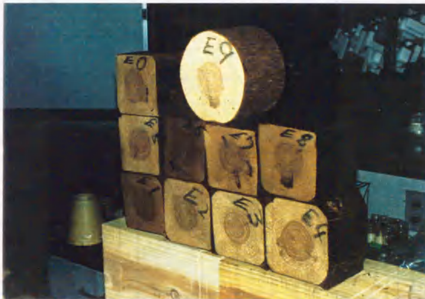
Fig. 1-3. Thinnings before and after compressive-molding.
