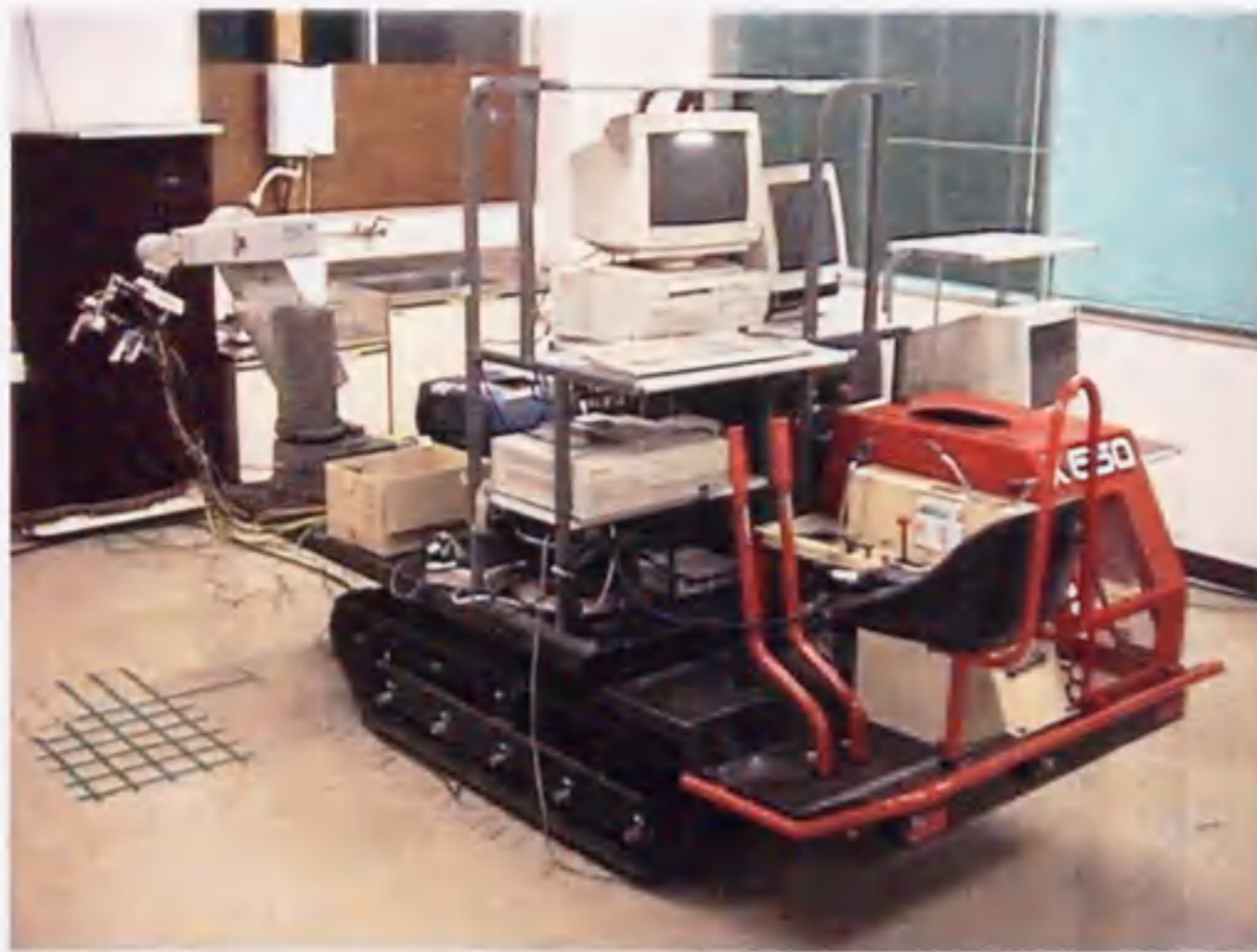
Fig. 4-3 General view of the robotic harvesting system for eggplants
