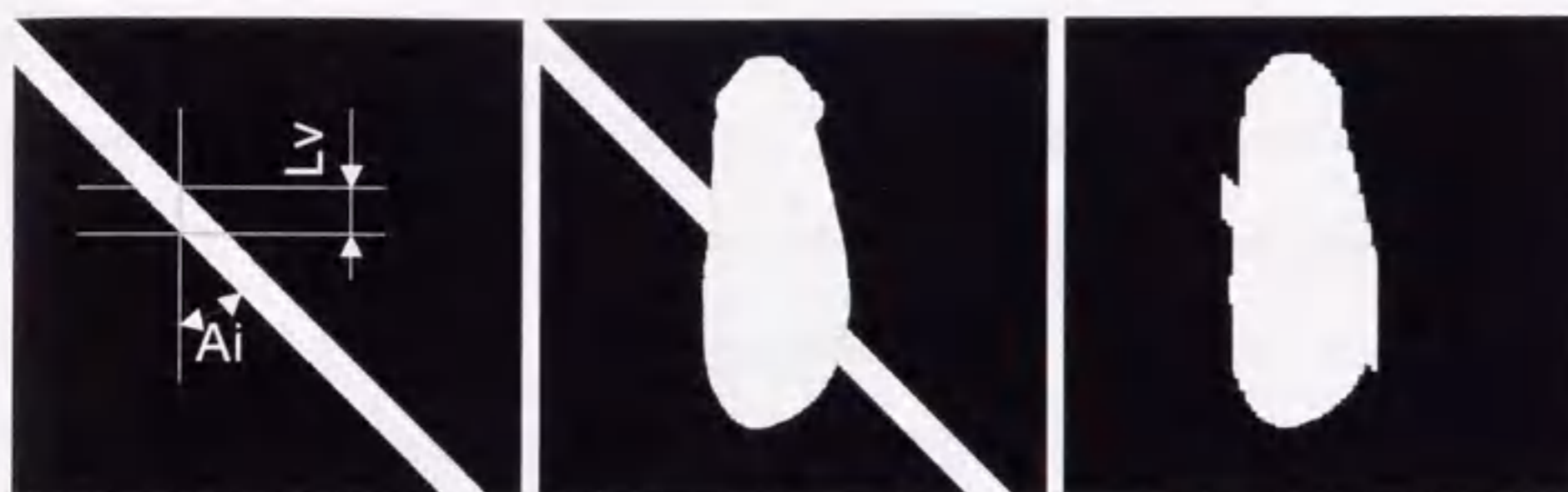
(a) Configuration of the diagonal line (b) Fruit binary image including stem (c) Final fruit binary image
