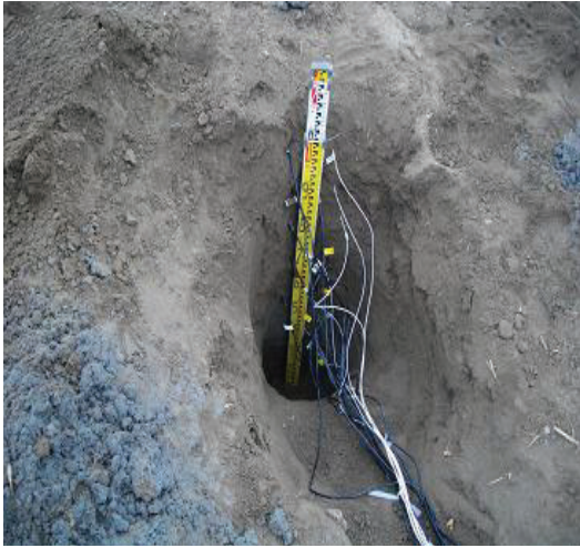
Fig 2.6-a Thermometer and TDR Sensor
