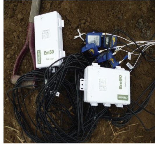
Fig 2.6-a Thermometer and TDR Sensor
