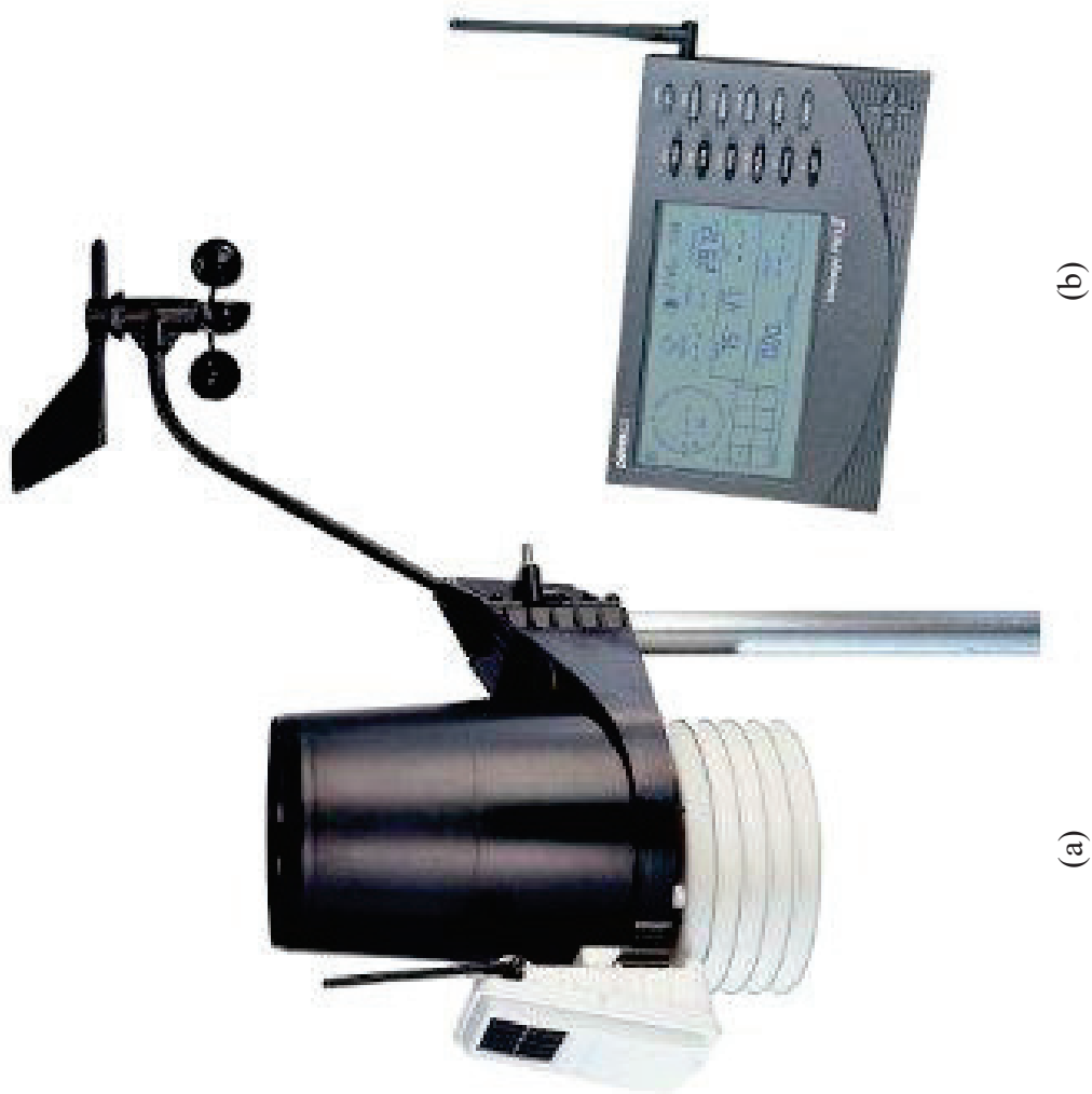
Figure 2.10 (a) Automatic Water Station instrument and (b) wireless data logger
