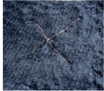
MFC anode – Carbon mat
