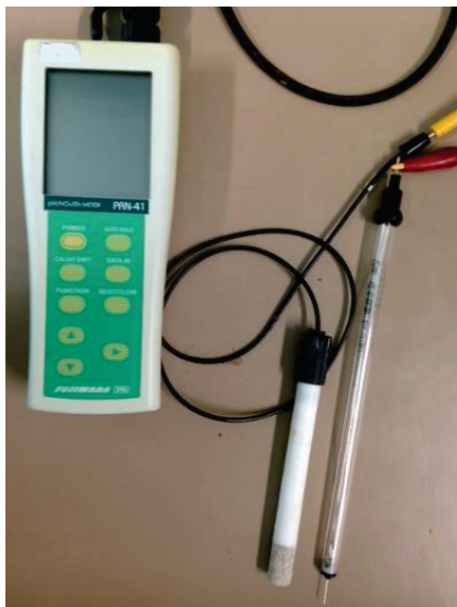
Eh meters (PRN-41; Fujiwara Factory Co., Ltd.)
