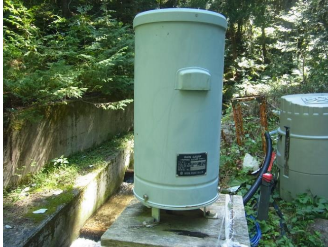
Fig.21 Tipping bucket rain gauge
