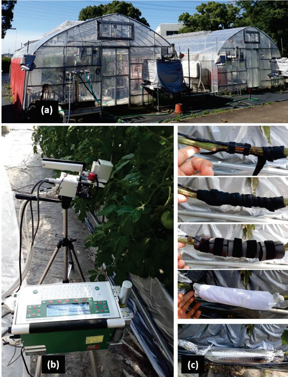
Fig. 4.1 (a) Naturally ventilated experimental greenhouse with CO 2 fertilizer (left) and without CO 2 supply (right); (b) photosynthesis measurement using a portable leaf chamber system (LI-6400, Licor, USA); (c) Dynagauge™ Sap Flow sensor installed on tomato stem that covered with the velcro strap, foam bodies, the white waterproof, and the bubble shield to prevent direct sunlight to sensor.
