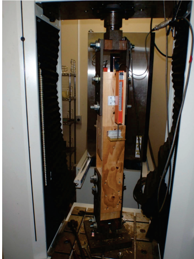
Fig. 4.2 State of specimen installation in the single shear test of joint
