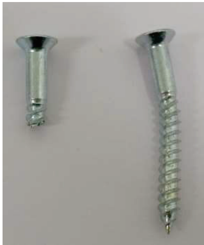
Fracture of fastener (right) Fastener bending yield (left)
