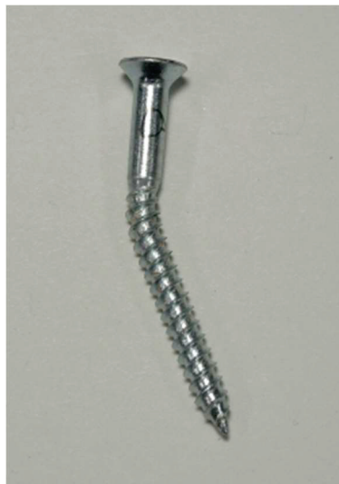
Fastener bending yield (4.5 × 50mm)
