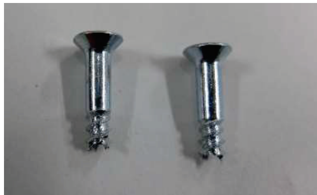
Fracture of fastener (4.1 × 38mm)
