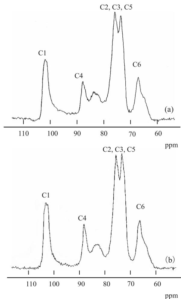
Fig. 5 CP/MAS  $^{13}\text{C}$ -NMR spectrum of paper yarn (a) untreated, and (b) high-pressure steamed at 180°C for 2 min. Letters show the carbon numbers of glucose unit.
