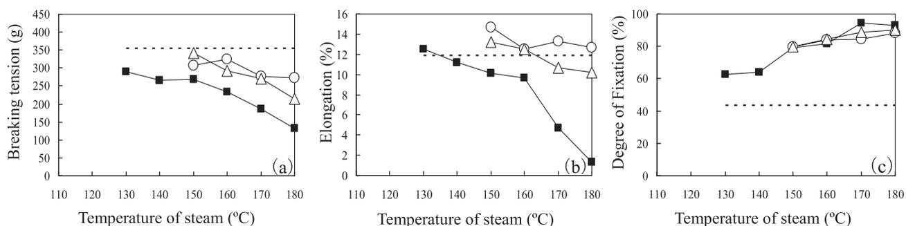
**Fig. 1** Physical property of 264 denier paper yarn treated by high-pressure steaming for 2 min. (a) strength, (b) elongation, and (c) degree of twisted fixation (■ : in dry condition, △ : in wet condition, ○ : in wet condition after soaking into 0.28 % NH<sub>3</sub> aqueous solution, --- : value before steaming).
