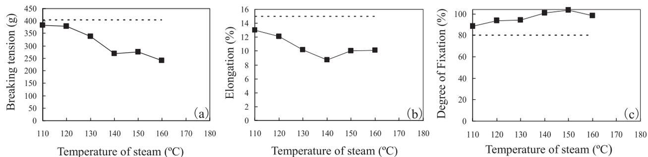
**Fig. 2** Physical property of paper/rayon yarn treated by high-pressure steaming for 2 min. (a) strength, (b) elongation, and (c) degree of twisted fixation (--- : value before steaming).
