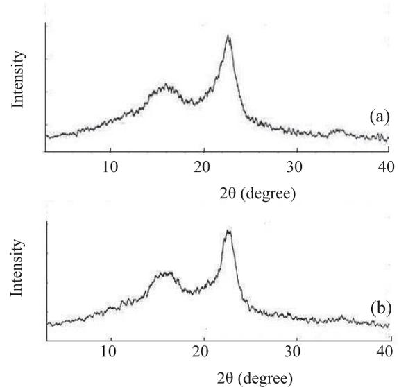
Fig. 4 X-ray diffraction of paper yarn (a) untreated, and (b) high-pressure steamed at 180°C for 2 min.
