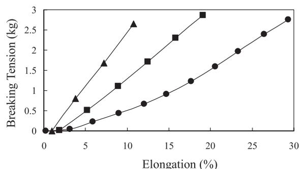
Fig. 3 The strength and degree of elongation of ten-twisted paper yarns (▲ : without twist, ■ : twisted at 150 r/m, ● : twisted at 400 r/m).
