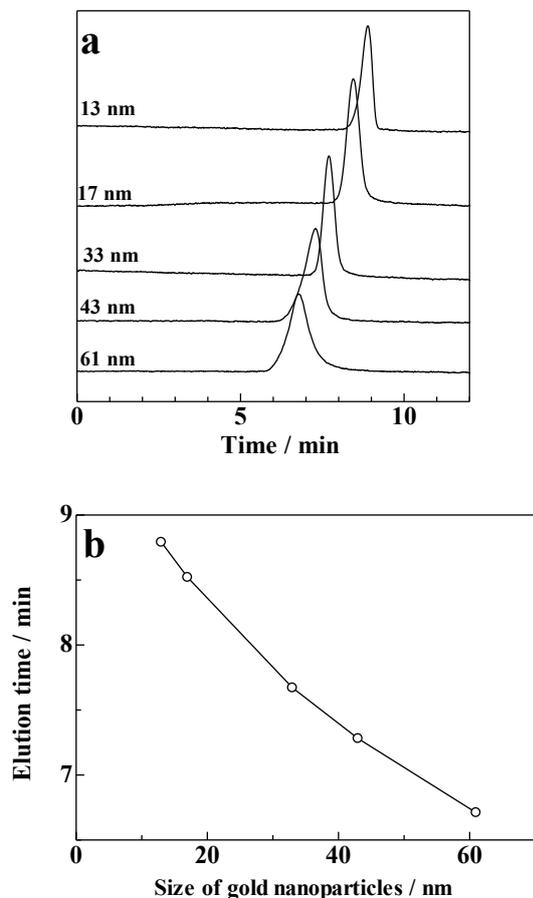
Fig. 6 Elution profiles of gold nanoparticles with different sizes (a), and the elution time as a function of the gold nanoparticle size (b). Column, monolith ( $400 \times 0.050$  mm i.d.); sample volume, 20 nL; wavelength of detection, 530 nm; mobile phase, 8 mM SDS; flow rate,  $0.1 \mu\text{L}/\text{min}$ .
