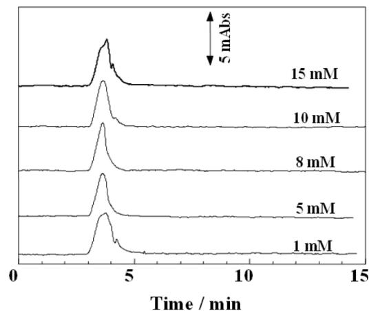
Fig. 5 Elution profiles of gold nanoparticles for aqueous SDS solution as the mobile phase. Mobile phase, aqueous SDS solution with different concentrations as indicated; analytes, 61 nm gold nanoparticle; other operating conditions were the same as in Fig. 4.
