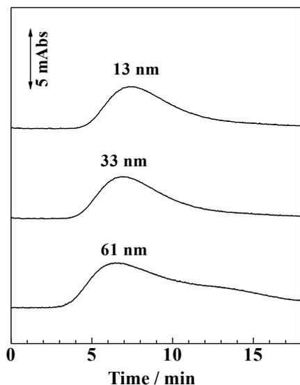
Fig. 4 Elution profiles of gold nanoparticles for water as the mobile phase. Column, monolith ( $200 \times 0.050$  mm i.d.); mobile phase, water; analytes, 13, 33 or 61-nm gold nanoparticles; sample volume, 20 nL; flow rate,  $0.1 \mu\text{L}/\text{min}$ ; wavelength of detection, 530 nm.
