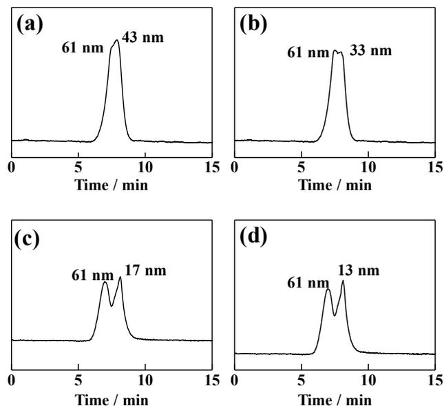
Fig. 7 Separation of gold nanoparticle mixtures on a 400-mm column. Samples, 43 and 61 nm for (a), 33 and 61 nm for (b), 17 and 61 nm for (c), 13 and 61 nm for (d), other operating conditions were the same as in Fig. 6.
