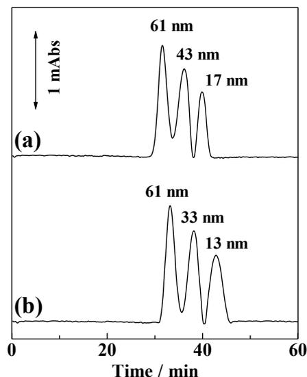
Fig. 10 Separation of gold nanoparticle mixtures on a 2000-mm column. Column, monolith (2000  $\times$  0.050 mm i.d.); analytes, 61, 43 and 17 nm (a) and 61, 33 and 13 nm (b); other conditions were the same as in Fig. 6.
