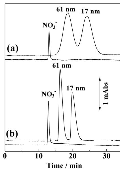
Fig. 8 Separation of gold nanoparticle mixtures on monolith columns with different mesopore growing steps. Columns, monolith with a mesopore growing step (a) or without any mesopore growing step (b),  $1000 \times 0.050$  mm i.d.; analytes, gold nanoparticles for the upper trace and 1 mM sodium nitrate for the lower trace; other conditions were the same as in Fig. 6.
