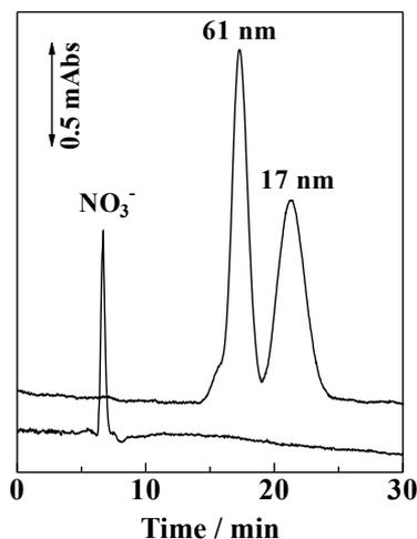
Fig. 9 Separation of gold nanoparticle mixtures on a packed column. Column, Hipresica FQ N2N (1.9  $\mu\text{m}$ , 100  $\times$  0.32 mm i.d.); analyte, 61 and 17 nm; sample volume, 0.2  $\mu\text{L}$ ; wavelength of detection, 530 nm; mobile phase, 8 mM SDS; flow rate, 0.5  $\mu\text{L}/\text{min}$ ; analytes, gold nanoparticles for the upper trace and 1 mM sodium nitrate for the lower trace.
