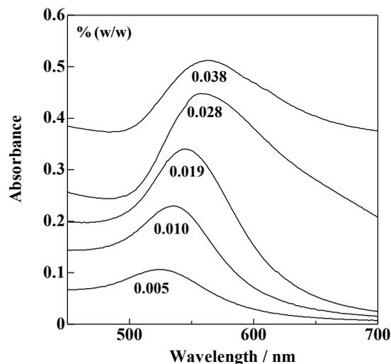
Fig. 1 UV-VIS spectra of gold nanoparticles for various volumes of  $\text{HAuCl}_4$ .
