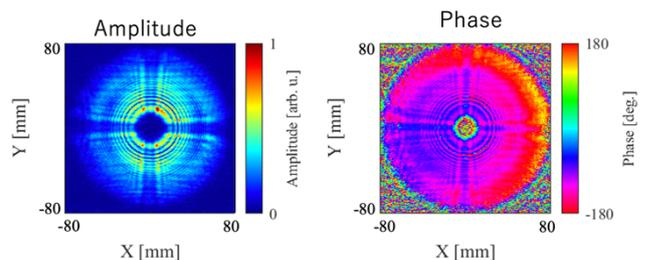
Fig. 2. Measured near-field distribution of the Cassegrain antenna at 300 GHz.
