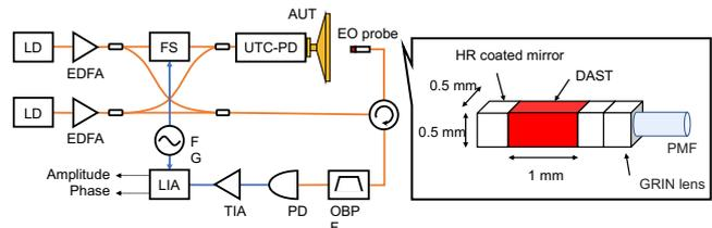
Fig. 1. Measurement setup and EO probe
